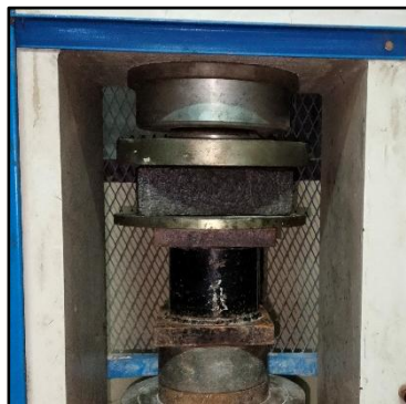
Gambar 2 Proses pengujian kuat tekan paving block
