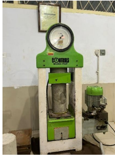
Gambar 1 Alat Kuat Tekan ( Compression Machine )
