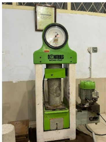
Gambar 1 Alat Kuat Tekan ( Compression Machine )
