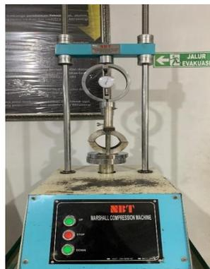
Gambar 1 Alat Marshall Test
