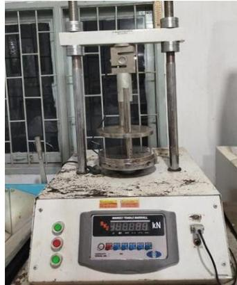
**Gambar 2 Alat Indirect Tensile Strength**
