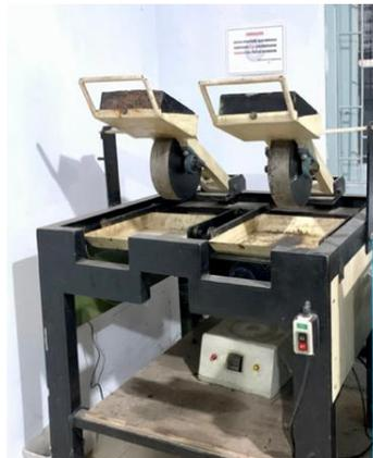
**Gambar 1** Alat Wheel Tracking Machine
