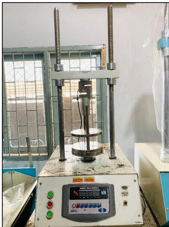
Gambar 1 Alat *indirect tensile strength*
