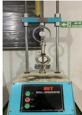
**Gambar 1** Alat *Marshall Test*
