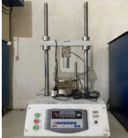
**Gambar 2 Alat Indirect Tensile Strength**
