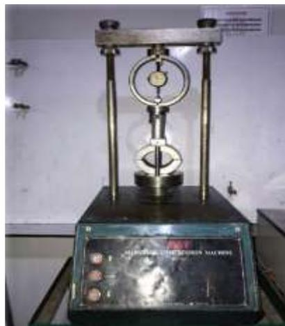
Gambar 1 Alat Marshall test
